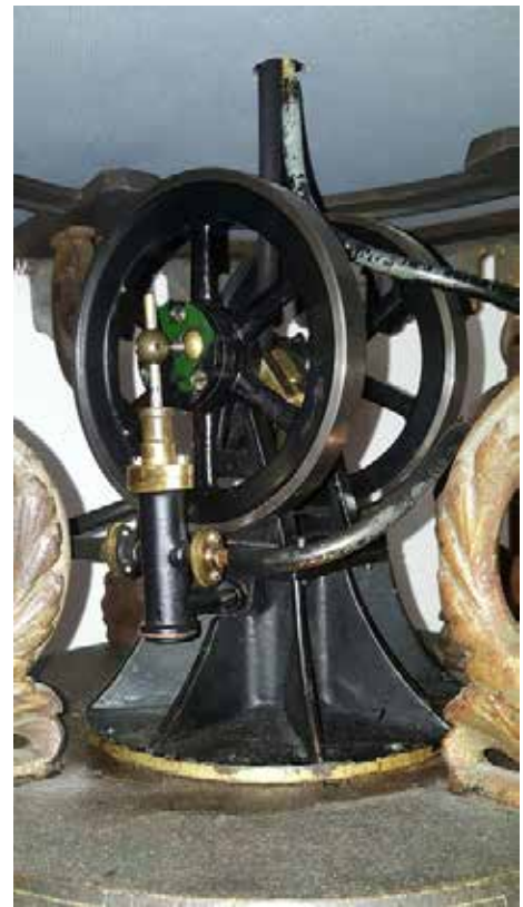
Raab air-cooled two-cylinder pumping engine. Note the big "cooling fins", a Raab's motors signature detail.
