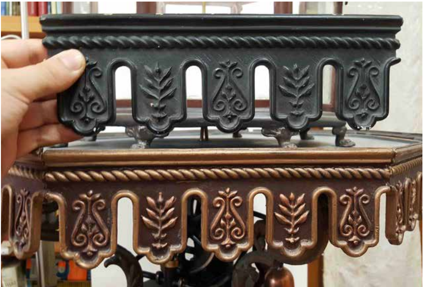
Building lambrequin -style replacement parts.
