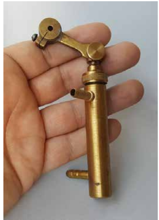
The Heinrici electric motor was equipped with a very small and elegant water pump.
