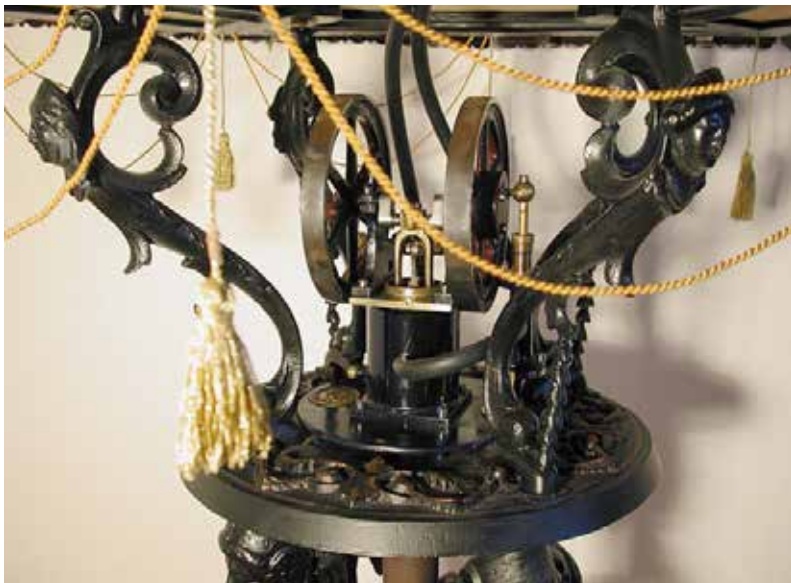
Heinrici water-cooled single-cylinder pumping engine.
