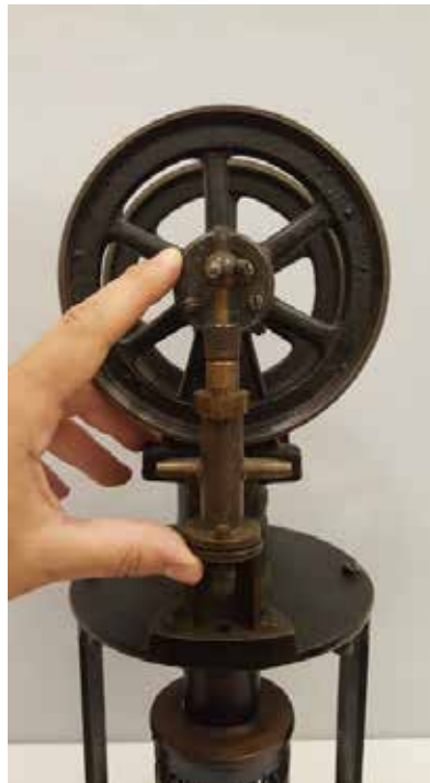
A classic example of water pump for two-cylinder hot air engines.
