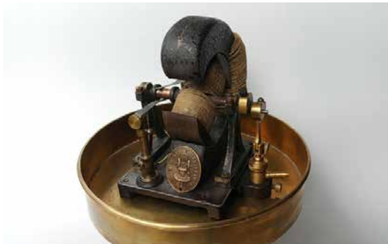
Heinrici electric motor designed for the model No. IIIA.
