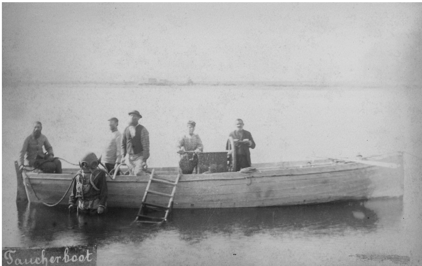
The diver in shallow water, 1890. Notice the bulky manual air pump on the boat. ©Stazione Zoologica Anton Dohrn, Archivio Storico (ASZN, La 126.14.).
