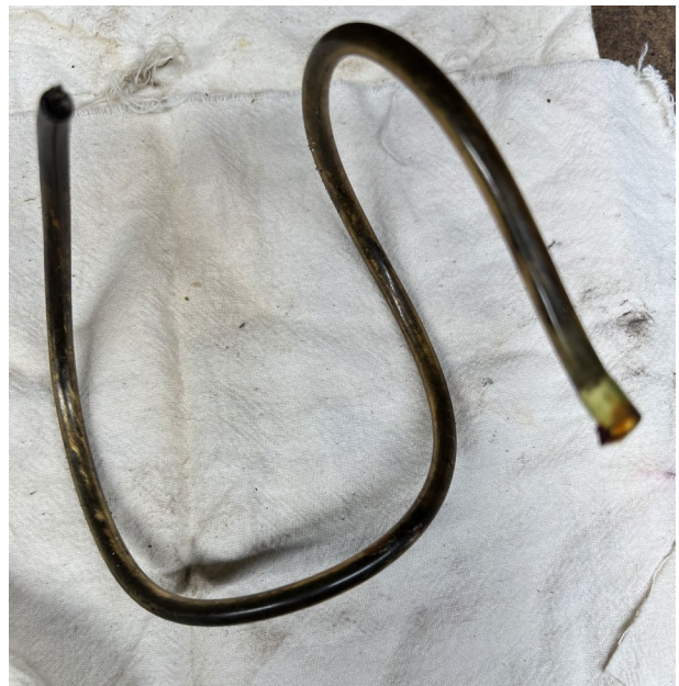
Figure 28 Clogged muffer hose
