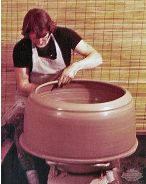
Making the front rim. The front viewing port on the aquarium is turned back on itself to create a flat receiver, where the glass will be attached. Photo courtesy of Robert Compton.
