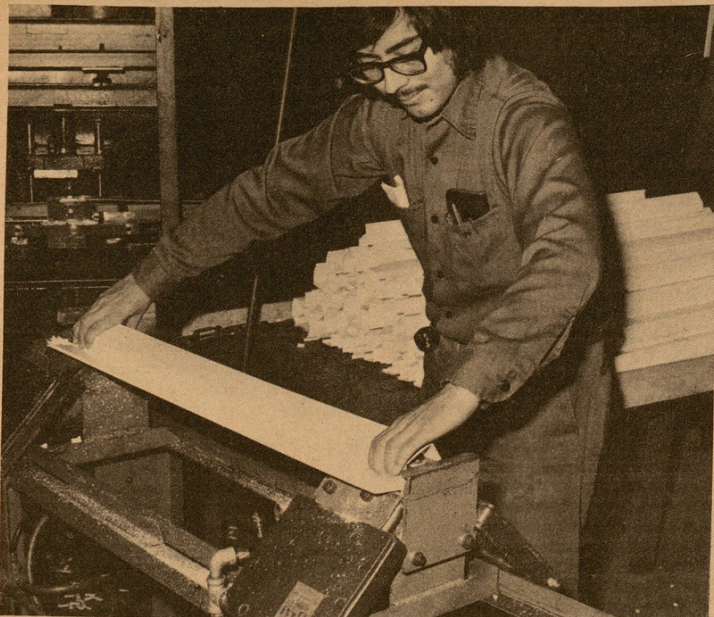
Polo-Lights are preformed then trimmed on a special cutter and assembled by hand. Fitted with fluorescent tubes they have become a popular product.
