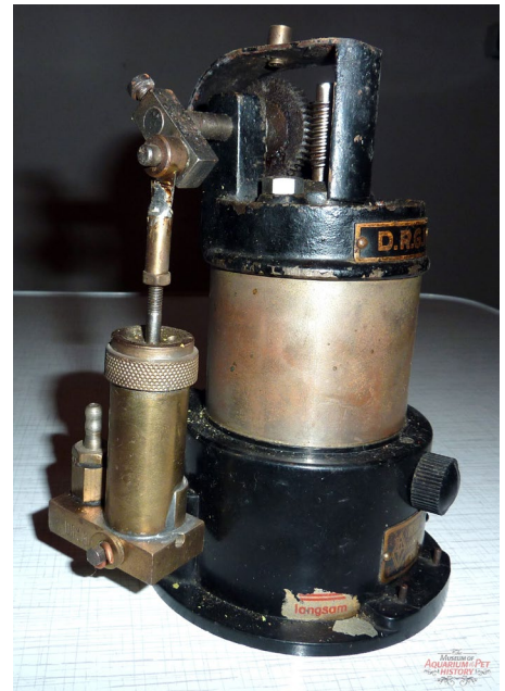
220-volt electric pumps used in aquaristics.
