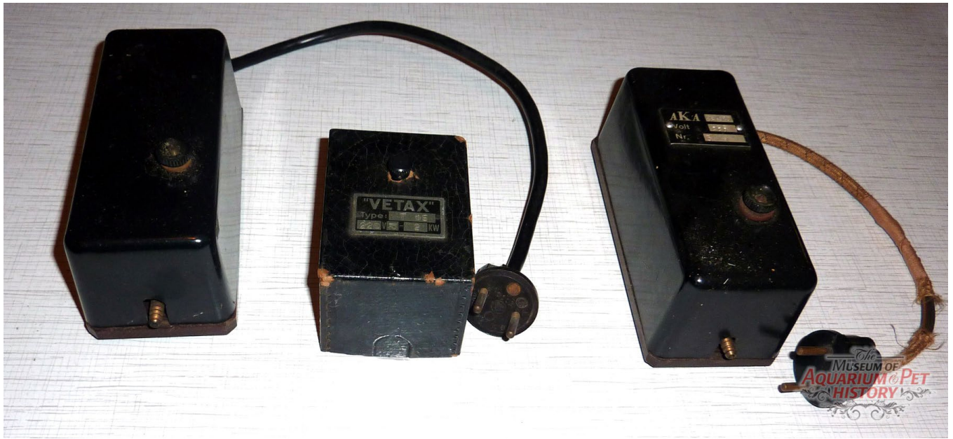
Membrane pumps from various manufacturers.
