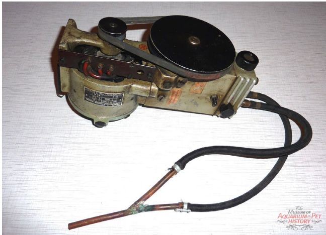
Membrane pump from the first half of the last century.
