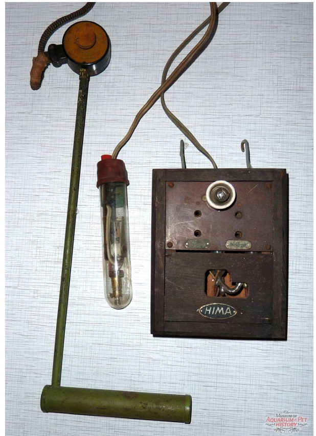
110-volt DC heater with relay.
