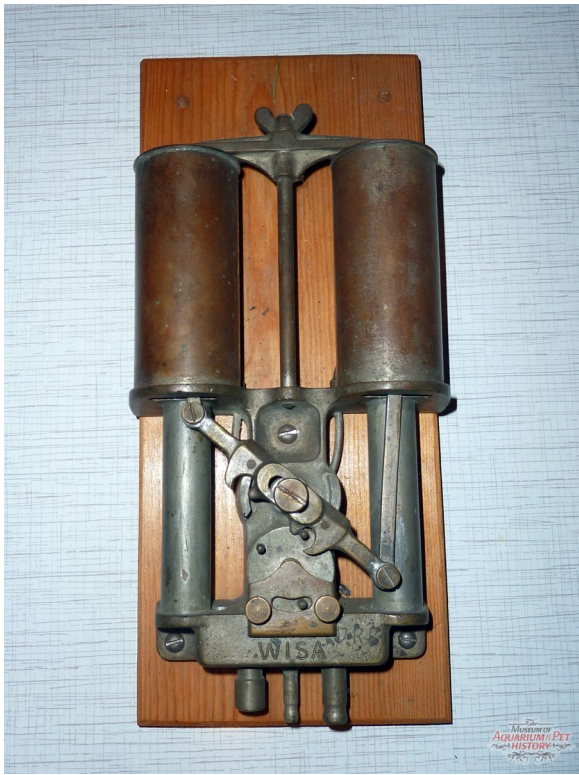
German-made air pump from the 1920s.
