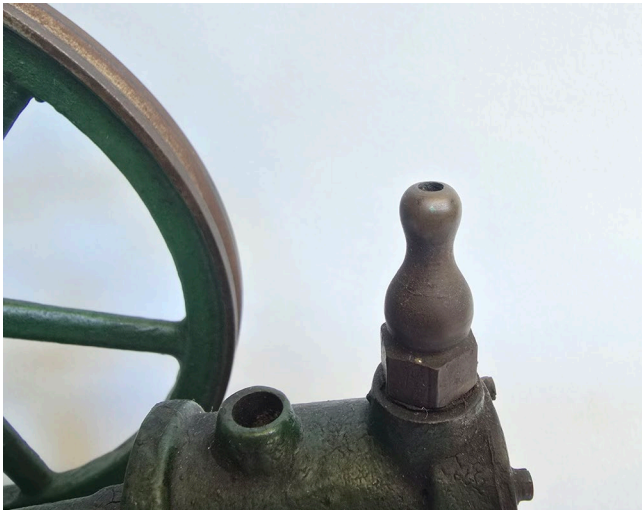
Close-up of the brass air outlet barb.
