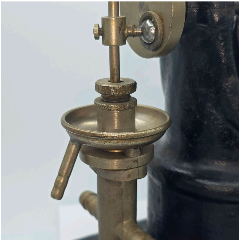
The brass drop-catcher mounted below the bushing.
