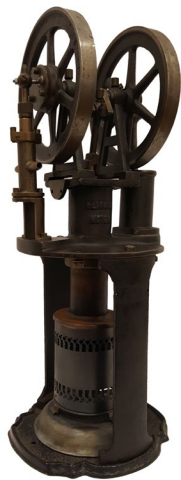
Double cylinder pumping engine by Louis Heinrich.
