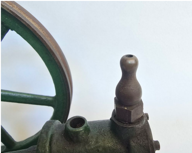
Close-up of the brass air outlet barb.
